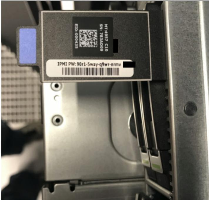
Figure 3-2 Hard disk drive pull-out tab
